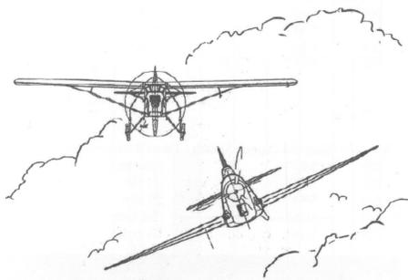
The two ships that are compared here show high performance "figures of merit" in most studies. They are the Curtiss Robin & Caudron C- 460 Racer. The Caudron is usually rated slightly higher, probably because of it's long nose, good tail moment and clean lines. The Robin has good proportions as well, but is at the other end of the spectrum regarding streamlining. The Robin does have one very important performance enhancing feature: an under-cambered wing.
