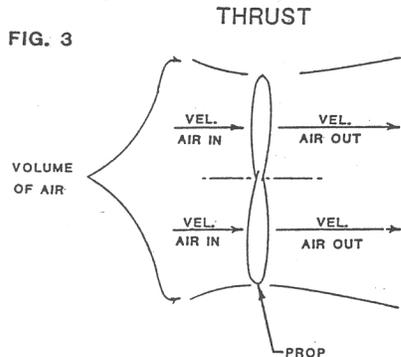
THRUST = VELOCITY OF AIR OUT MINUS VELOCITY OF AIR IN
